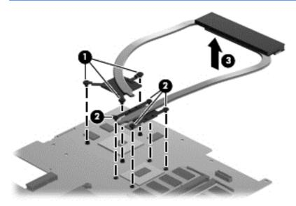
b. Thoroughly clean the thermal connections (1), (3) on the system board and the heat sink (2), (4) before replacing a heat sink onto a system board. Continue to step 3.
